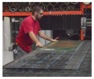
Here at <u>Elasto Proxy</u> (Boisbriand Quebec, Canada), our water jet cutting machine uses Ingersoll-Rand highpressure heads that direct jets of 50,000 pounds per square inch (psi) towards an X-Y axis table with a 5' x 10' cutting surface.
